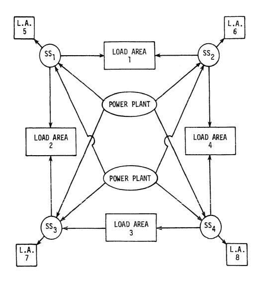
Figure 3.1. Electrical supply system
