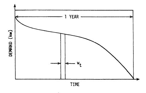
Figure 3.3. Load duration curve
